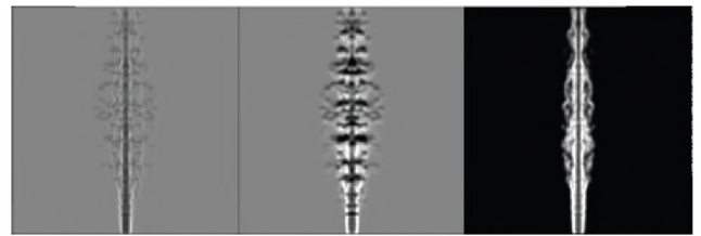
Figure 8: Results of a combustion dataset of dimensions 480x720x100 seen in figure 6 rendered with 10 iterations of progressive refinement per frame using cone filtering on a Geforce GTX 280 card at 512x512 resolution.
