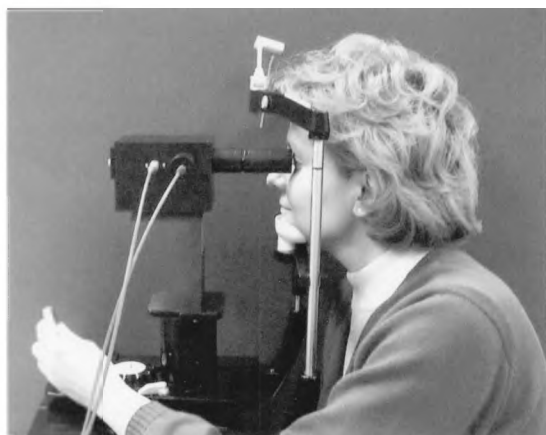
Fig. 5 Measuring MP level. The subject looks into the instrument and adjusts the optical alignment while resting the forehead against the device.
