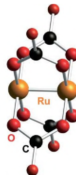
1 , Paddle wheel-structured ruthenium acetate, \text{Ru}_2(\text{O}_2\text{CMe})_4 (Hs not depicted)
