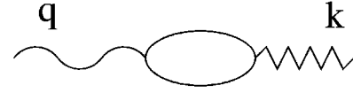
FIG. 4. Transition amplitude for the direct conversion of the electric field (wavy line) to a phonon (zigzag line). The loop stands for the electron polarization operator \chi(\omega, q) .
