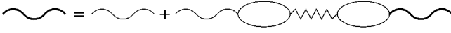
FIG. 1. The Dyson equation for the propagator of the scalar potential (shown by the bold wavy line) in the lowest order in the electron phonon interaction. The thin wavy line stands for the propagator evaluated in the conventional RPA approximation, U(\omega, q) = V_q / [1 - V_q \chi(\omega, q)] , the zigzag line represents the phonon Green function, the loop stands for the electron polarization operator \chi(\omega, q) .
