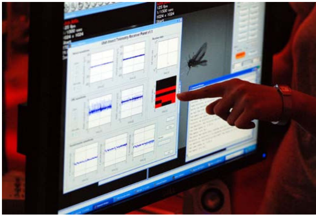
Figure 8. Photograph of live wireless data acquisition from locust flying in wind tunnel. Wing beats are visible in EMG traces (center, left of finger). High-speed video of locust is synchronized to telemetry data.
