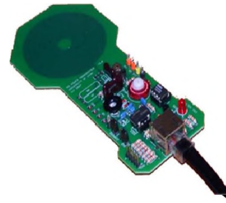
Fig. 4. Power and command transmitter with an integrated PCB coil in a diameter of 5.8 cm. The coil is driven at 2.765 MHz to provide power and a clock signal to the INI4 chip, and the amplitude of this signal is modulated to send commands to the chip.
