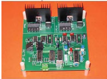
Fig. 13. The experimental prototype of the P-cell and N-cell. The upper left section shows the P-cell, the upper right section shows an N-cell. The bottom part of the board shows the gate drive circuit.
