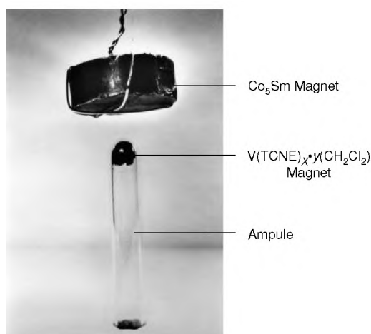
Fig. 3 Photograph of a powdered sample of 1a being attracted to a \text{Co}_5\text{Sm} magnet at room temperature
