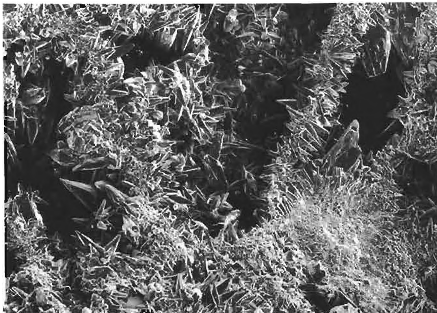
Figure 10. Sample 133-824A-10H-1, 79–80 cm; well-cemented sample showing poorly connected vugs and substantial recrystallization that blocks pore throats.
