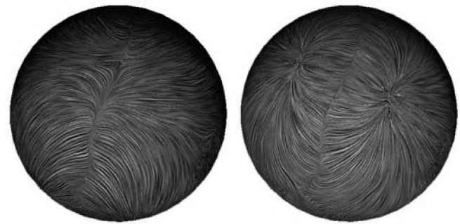
Fig. 14. Time-dependent sphere data set visualization in GPUFLIC.
