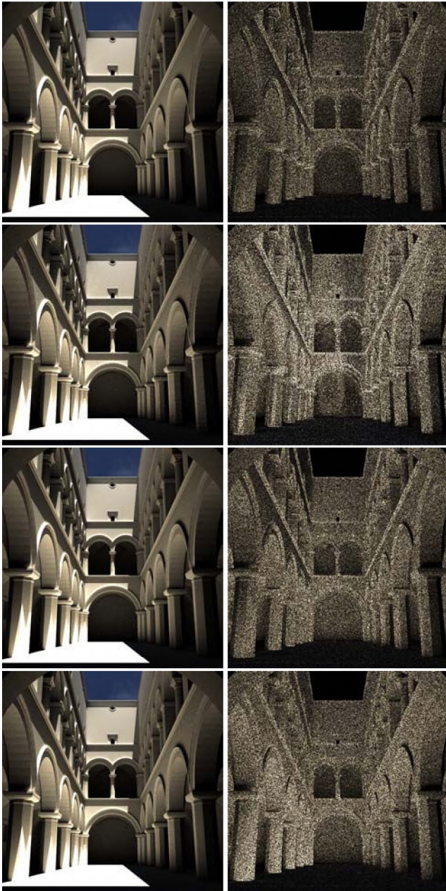
Figure 5: The Sponza Atrium illuminated by a directional light with 1-bounce global illumination, rendered using (from top to bottom) SMC importance sampling and control variates (1024 spp), SMC importance sampling alone (1066 spp), SMC control variates alone (1059 spp), MCMC BRDF importance sampling (1144 spp) all in 2.6 hours.
