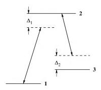
FIG. 1: A sketch of the atomic energy levels coupled to the coupling and probe fields.
