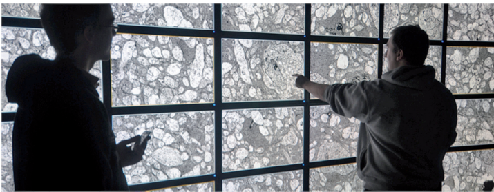
Figure 5. Visualization of the retina connectome dataset on a Powerwall with 24 30-inch monitors. The Visualization Streams for Ultimate Scalability (ViSUS) software system enables real-time management and visualization of very large datasets, such as 3D neural image volumes.
