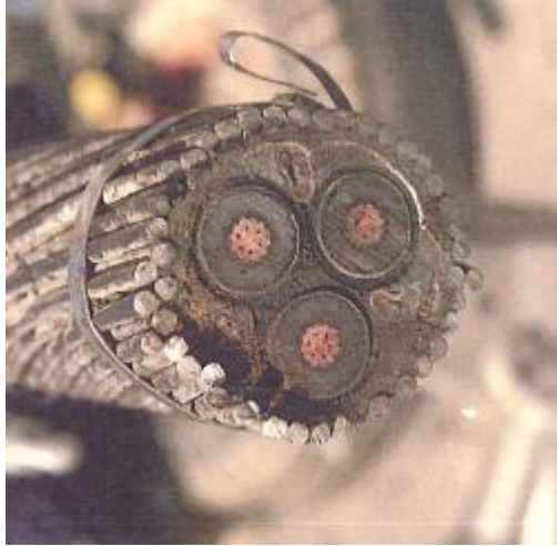
Fig. 8 3 core, 350 MCM sub sea cable
