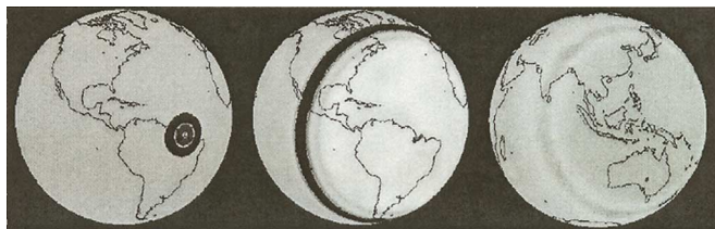
Fig. 2. Snapshots of impulsive wave propagation around the Earth as calculated by the 3-D FDTD model of [36] (the complete video can be downloaded at http://www.ece.northwestern.edu/ecefaculty/taflove/3Dmovietext@gif.avi ) (figure courtesy of [36]).
