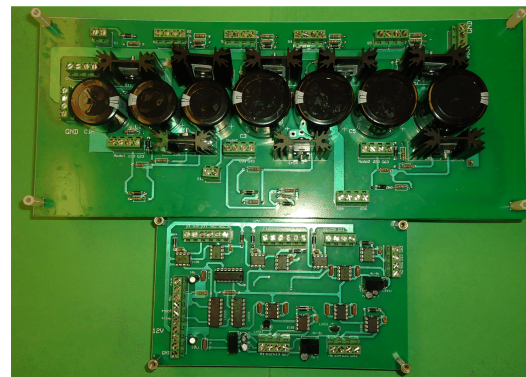
Fig. 10. Reconfigurable 5-module MMCCC prototype
