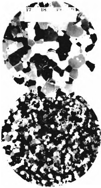
Figure 3. Examples of variable nature of grain size and texture in snow ice in Weddell Sea pack ice.
