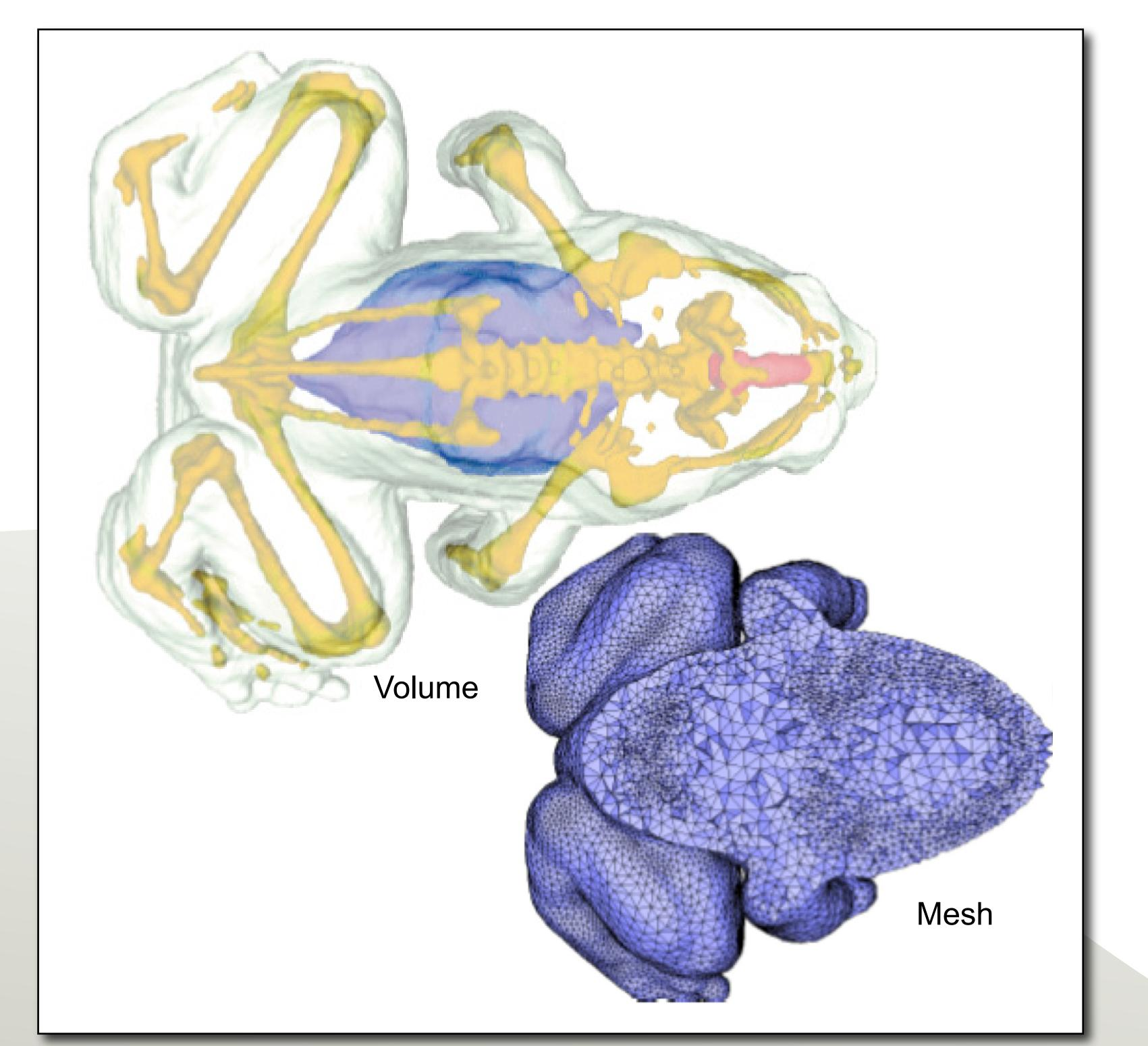
A meshing technique known as "Isosurface Stuffing" was created several years ago by Francois Labelle and Jonathan Shewchuck. The method involves laying volumetric data overtop a Body-Centered Cubic Lattice. This regular structure is made of cubes, with four tetrahedra spanning neighboring cubes. In this way, we only need to define rules to mesh a small number of cases of planes intersecting Lattice Tetrahedra. These cases can be quickly looked up, from a precomputed table.
