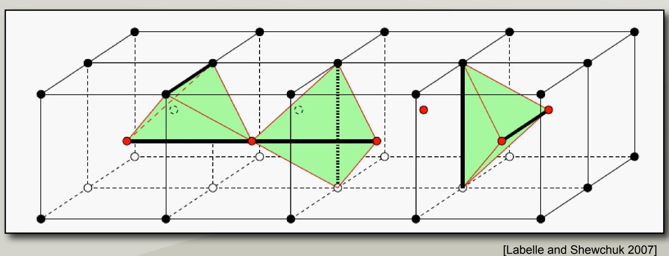
Whereas some meshing techniques can provide very high quality multimaterial meshes, they do so at consderaibly slow speeds. This 'stencil' based approach provides meshes at exceptionally fast speeds, with a tradeoff of decreased quality. For some purposes, a reasonable quality mesh made available immediately, is more useful than a high quality mesh available
