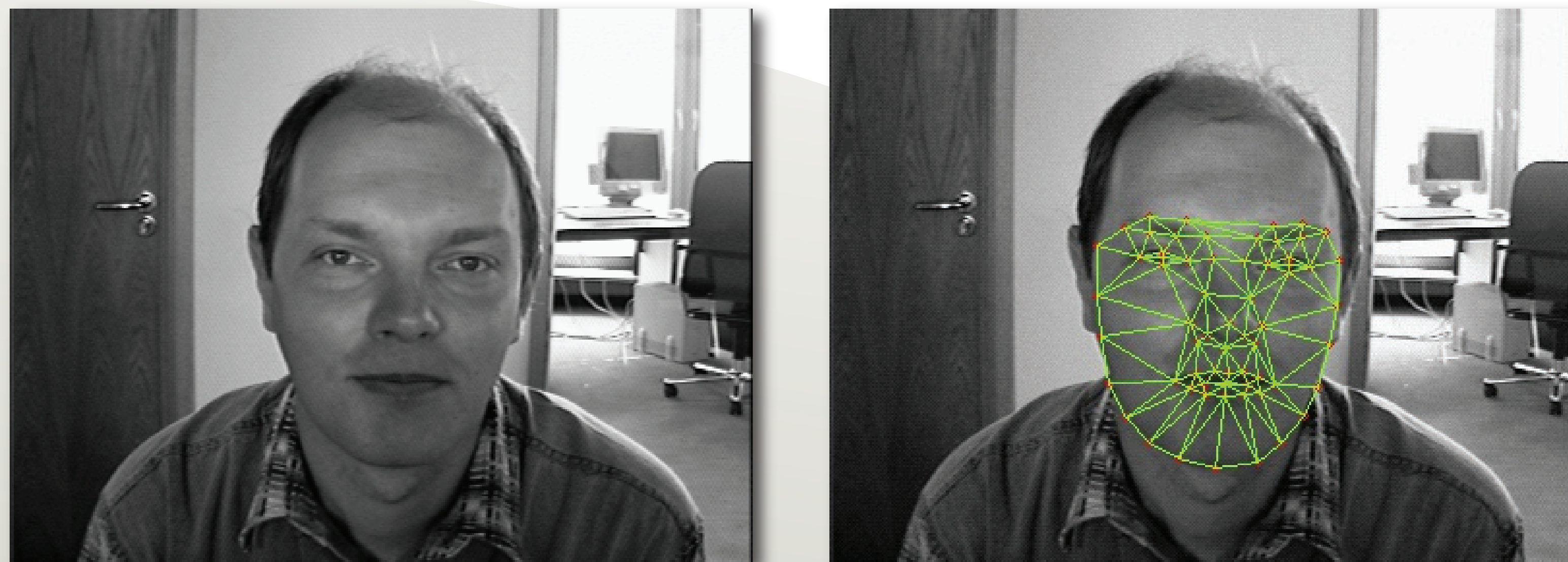
Figure 1. The first picture is original front face image and the second one is applied on Active Shape Model.
