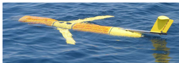
Fig. 9. Slocum Glider as used by the University of Southern California (courtesy of Smith et al. [47]).
