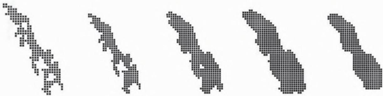
Figure 4: An example of a segmented region. The region after the hole filling algorithm has been run. The region after being grown, the region after having been shrunk.
