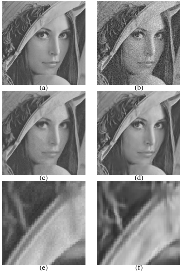
Figure 6. (a) Lena image (intensity range 0:100). (b) Noisy image (RMSE 10). (c) UINTA filtered image (RMSE 4.6). (d) Wavelet denoised [18] image (RMSE 3.6). (e) and (f) show zoomed insets of (c) and (d) respectively.
