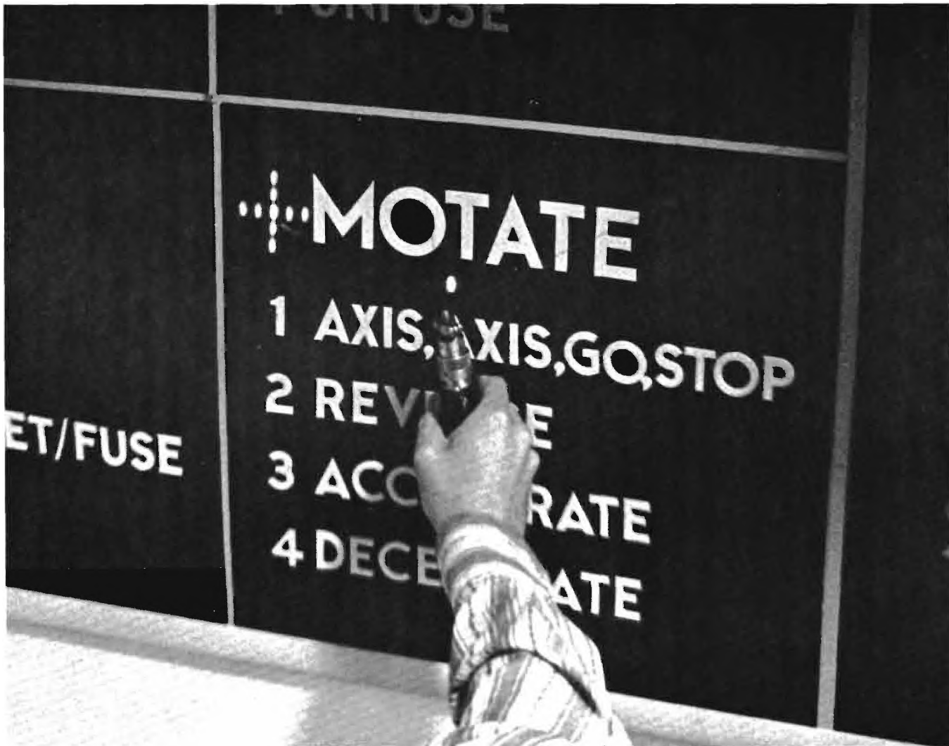
Fig. 11: Photograph of the wall chart taken through the head set. In addition to the observer's hand, the wand cursor and mode cross are visible.
