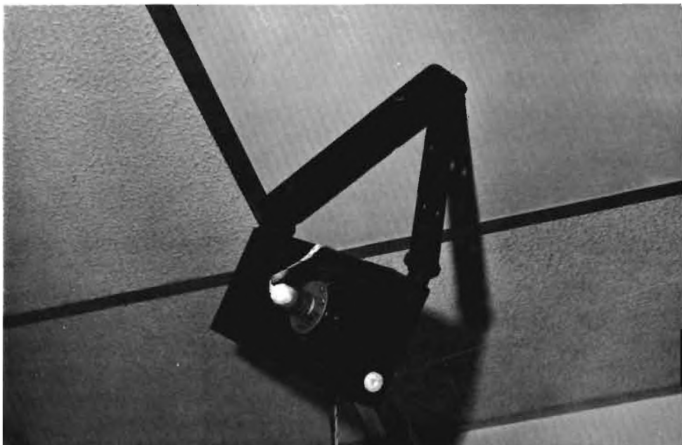
Fig. 10: One of three ceiling-mounted "puppet boxes." A monofilament line can be seen extending from a white teflon grommet. Protruding from one side of the box is a rotary pulse generator.
