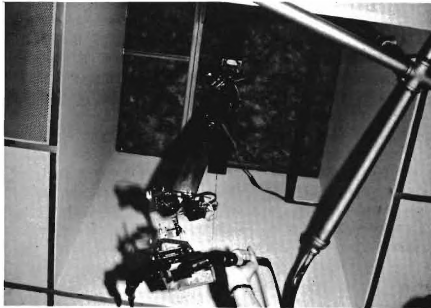
Fig. 7: Looking upward along the head position sensor shaft. The head set and a portion of the ultrasonic "shower stall" are also visible.
