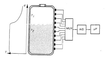
FIG. 2 - An Array Thermal Detector of Liquid Level
