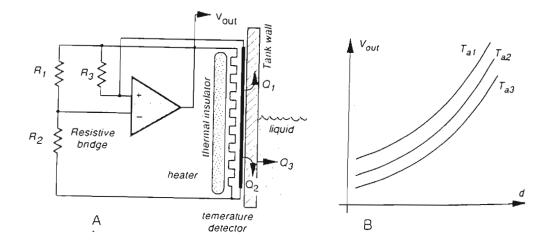
FIG. 3 - Active Thermoresistive Liquid Level Sensor A: Simplified Circuit Diagram B: Voltage Across Heating Elements For Three Different Tank Temperatures
