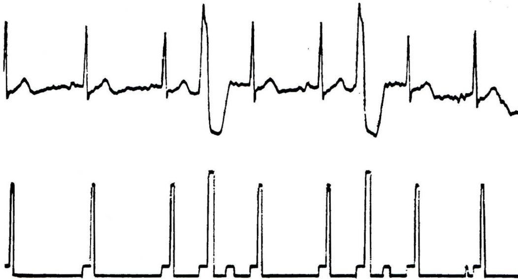
FIG. 7. Coded analog channel (lower trace) indicating computer decisions on QRS complexes (upper trace). Commencement of possible QRS indicated by small deflections. Recognition of normal QRS results in large deflection of fixed duration and height. Small deflections not culminating in QRS recognition signal are due to P or T waves and are excluded on basis of short duration. Detection of PVCs results in tall deflection of different height from normal. If criteria for PVC recognition are increased duration or combination of increased duration and prematurity the tall deflections are wider than normal (as in this record).
