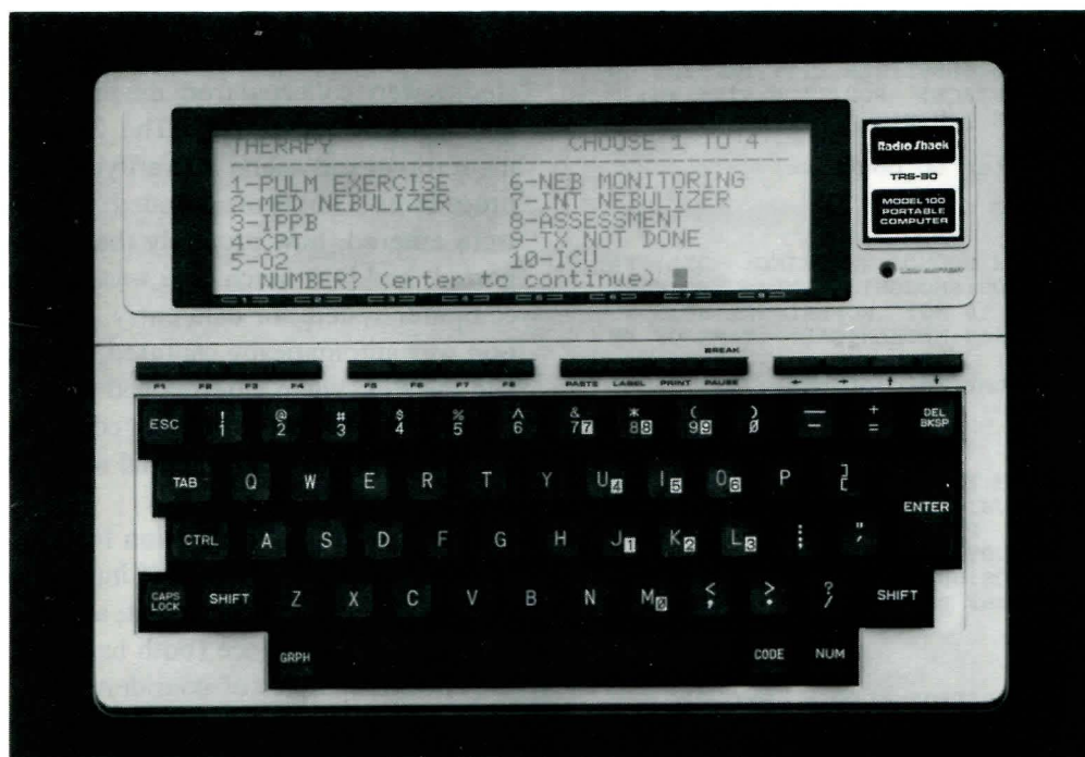
Fig. 1. Photograph of portable lap computer (PLC) used for charting respiratory care procedures.
