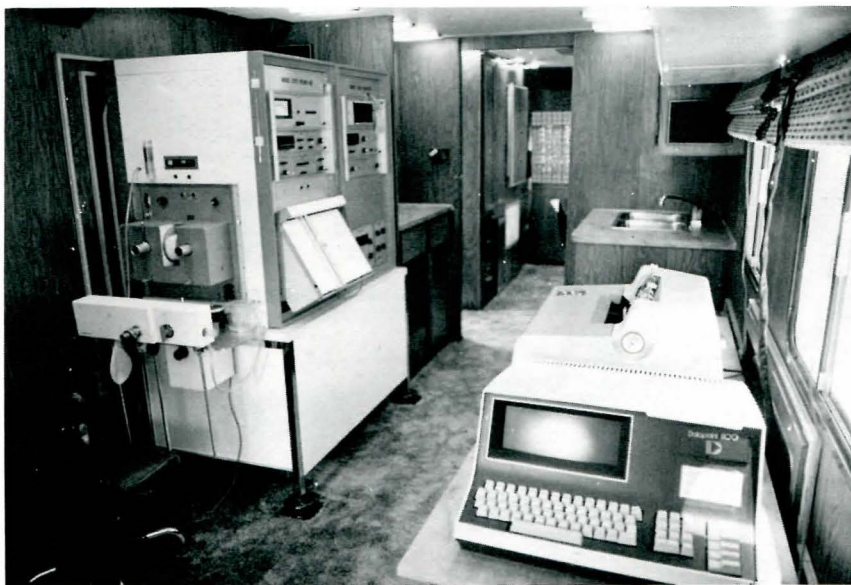
Figure 2 View toward rear of laboratory displays Pulmolab, CRT, and printer. Compartment behind Pulmolab can be used for exercise testing equipment or plethysmography. Rear of unit contains generator, refrigerator, head, water storage, filing cabinet, and voltage regulator. Driving area is used for administering the questionnaires.
