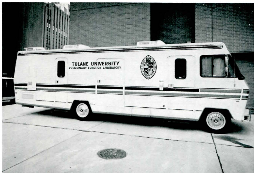
Figure 1 Exterior of mobile laboratory displays several access hatches and electronic leveling jacks. Test tanks are mounted on roll-out storage trays (not shown).
