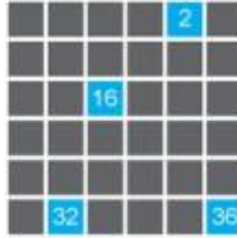
Figure 4.3: Illustration of a single township parcel in the state of Utah along with the four subdivided units given to the state.
