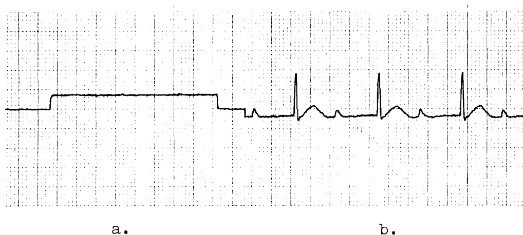
Figure 14. a. Compensated episode signal; b. Compensation of a simulated ECG signal. (25mm/sec., 1mv/cm)
