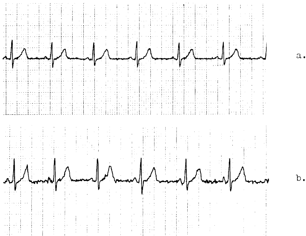
Figure 3. a. Original ECG signal; b. Compensated ECG playback waveform. (25mm/sec., a. 1mv/cm, b. 1mv/1.3cm)
