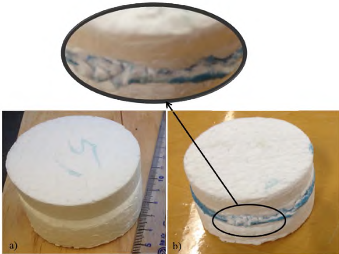
Figure 2.7. EPS specimens after direct shear testing: a) Intact and b) Glued
