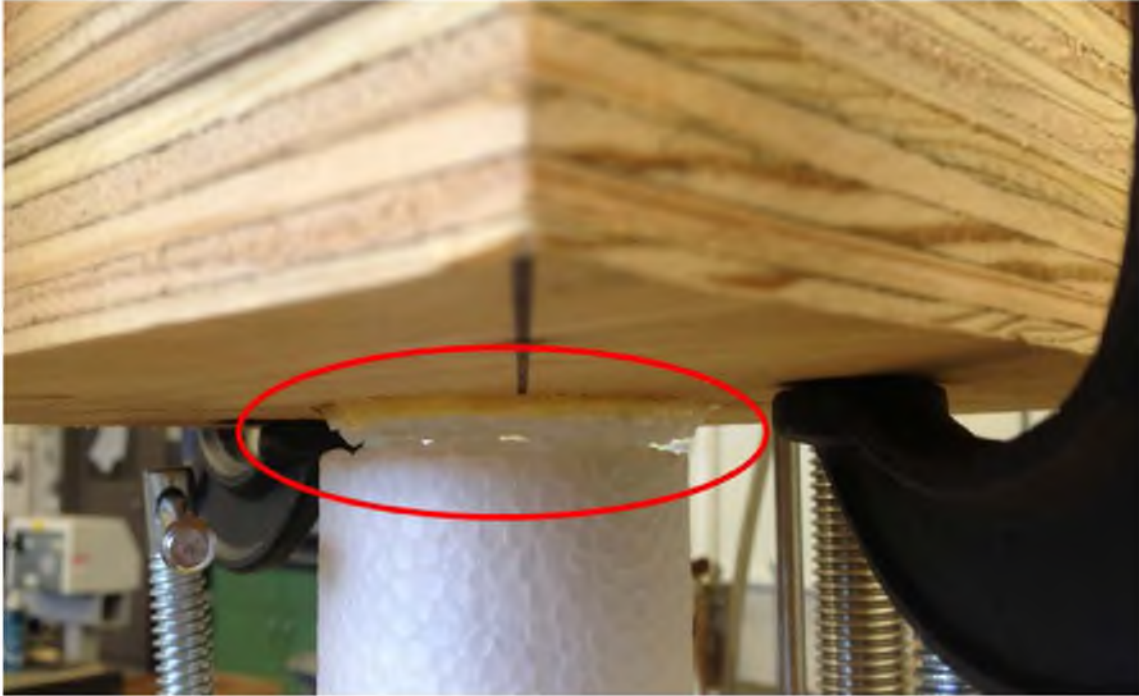
Figure 2.15. Tensile rupture in EPS geofoam specimen
