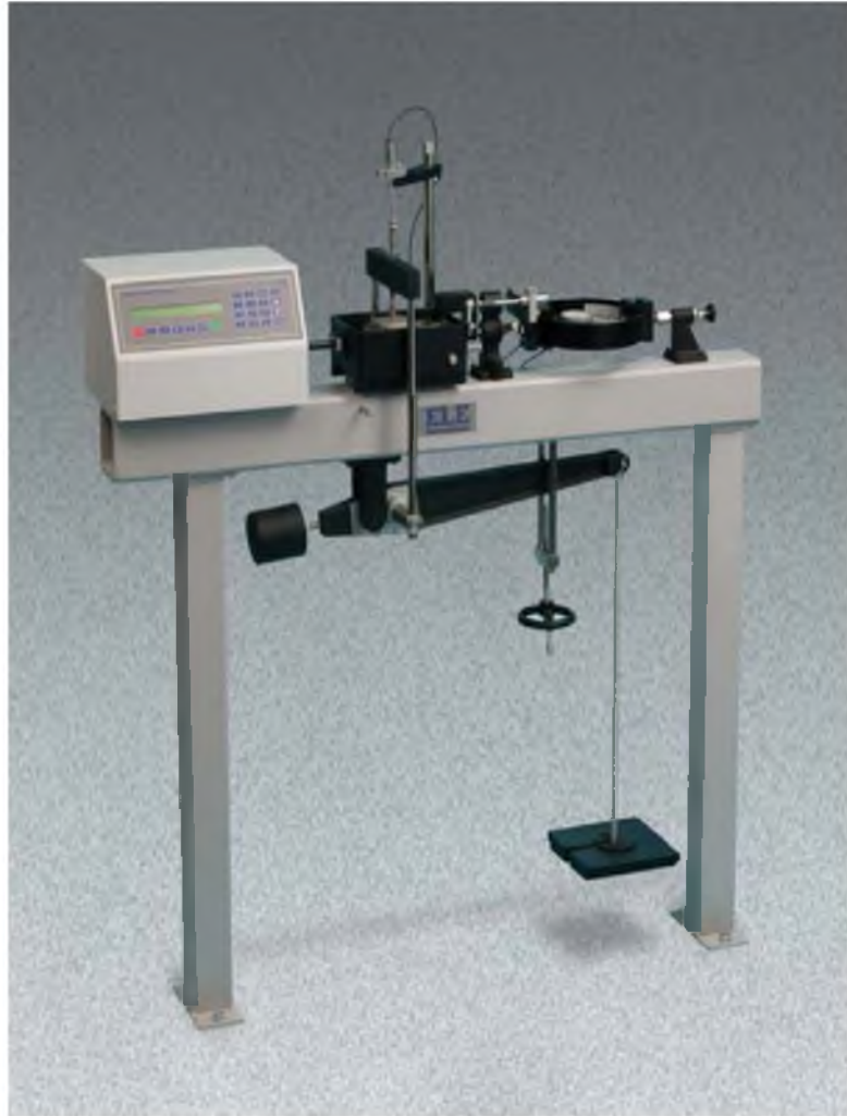
Figure 2.6. University of Utah direct shear device manufactured by ELE International
