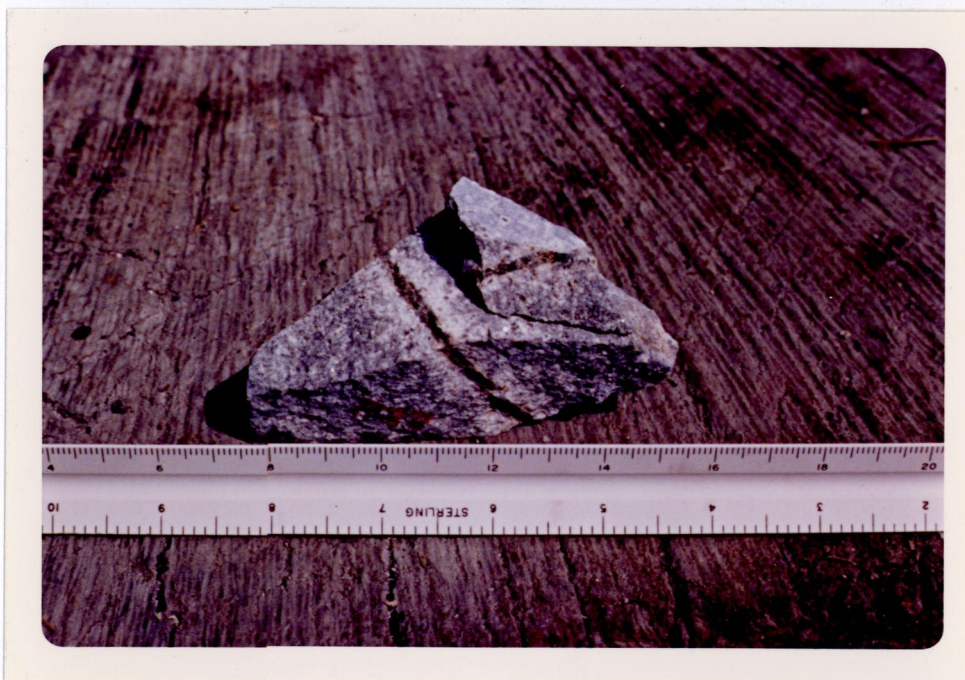
Fig. 6.- Veinlet of garnet and other minerals in porphyry.
