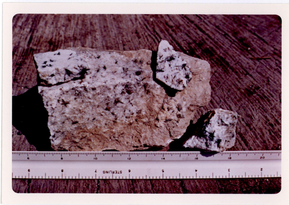
Fig. 16.- Ludwigite in recrystallized limestone (calcite) from (800S, 800W) (pl. 1).
