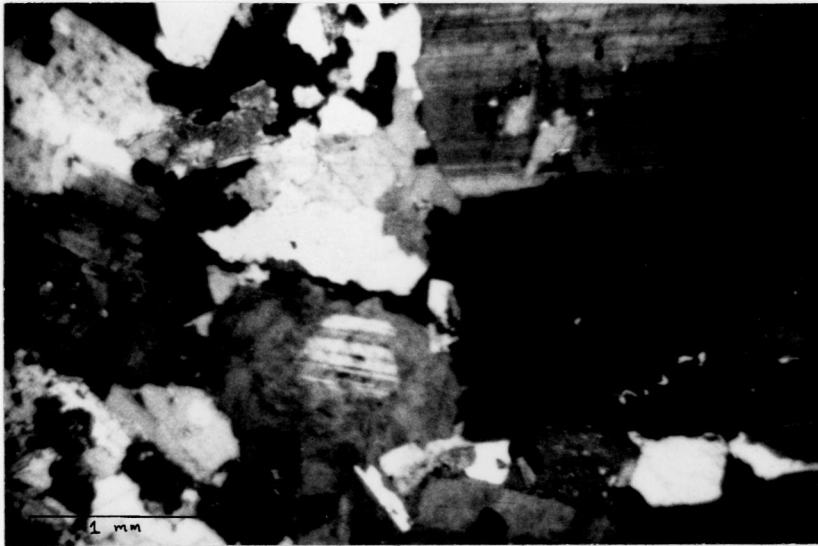
Fig. 3.- Photomicrograph of the quartz monzonite porphyry.
