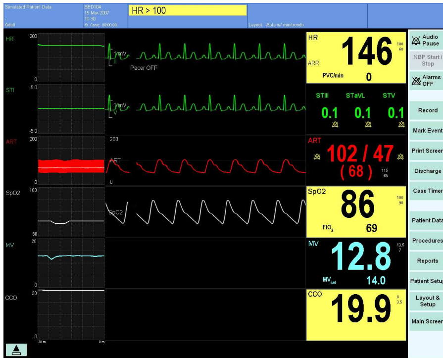
Figure 5.3: Control display consisting of a Dräger Kappa XLT patient monitor and an Alaris Medley infusion pump. The display is presenting a patient with multiple alarms: high heart-rate (HR), low blood oxygen saturation (SpO 2 ) and high cardiac output (CCO). Three infusion pumps are currently running.
