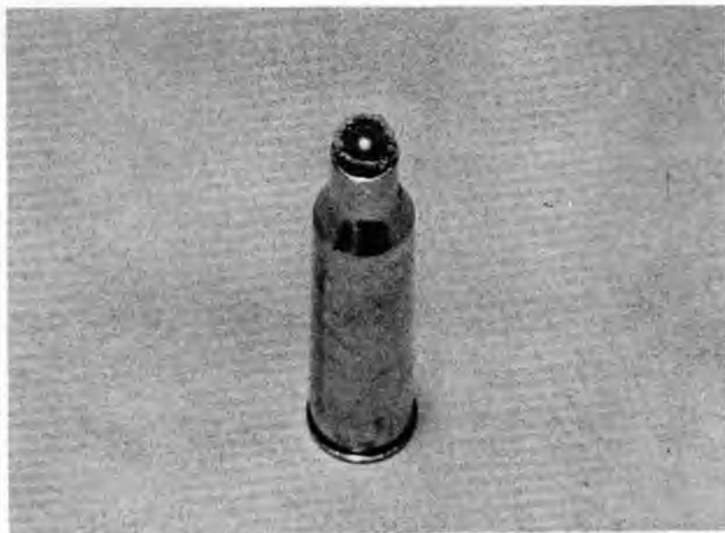
Fig. 4. Swift cartridge with sabot and copper sphere. All cartridges used in this research were filled with 2\ 1/2 cc of 2400 Hercules Smokeless Powder and 1/2 cc of 4064 DuPont Rifle Powder in that order.
