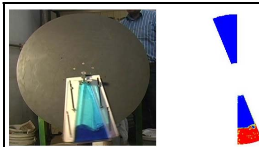
Figure 5.16 – Experimental and CFD discharge profiles for 85% by volume glycerol solution
