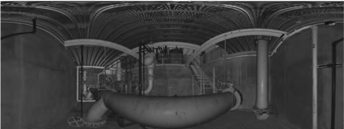
Figure 1-2 Measured brightness data acquired by a LiDAR scanner
