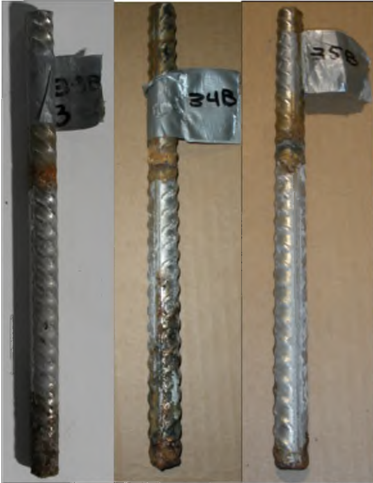
Figure 35 Ternary SSC (end cut) after impressed current test
