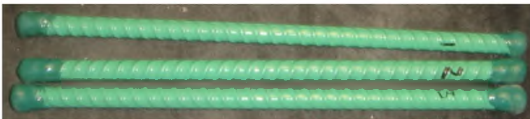
Figure 6 Undamaged ECR bars
