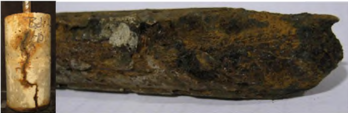
Figure 33 SSC bar (pinhole) in OPC after impressed current test
