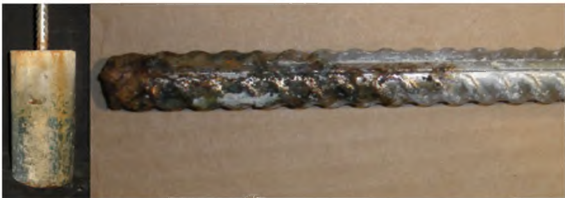
Figure 36 SSC bar in ternary (end cut) after impressed current test
