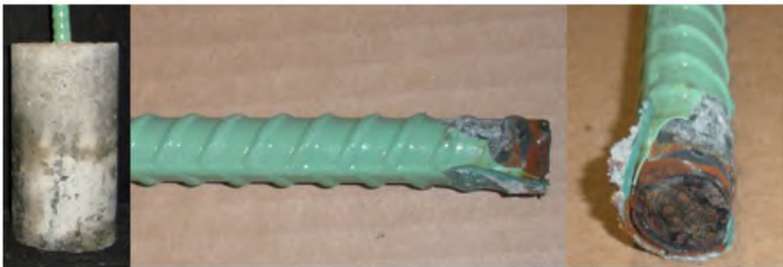
Figure 45 ECR (endcut) in ternary after impressed current test
