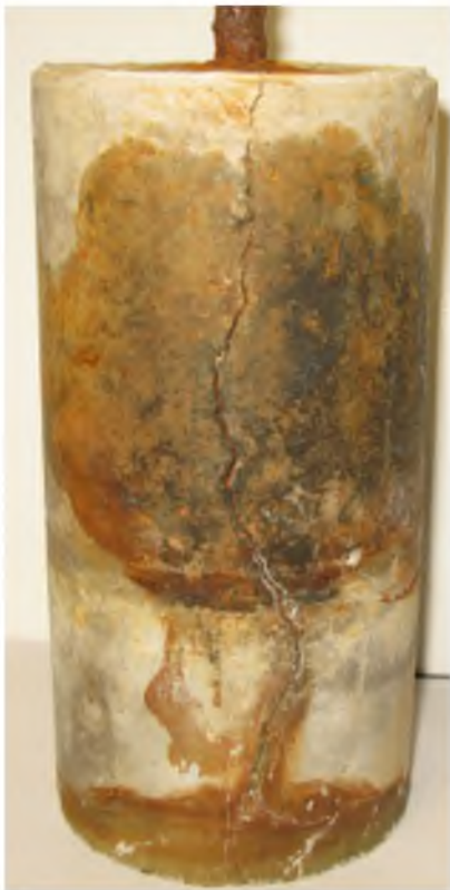
Figure 19 Black bar in OPC after impressed current test
