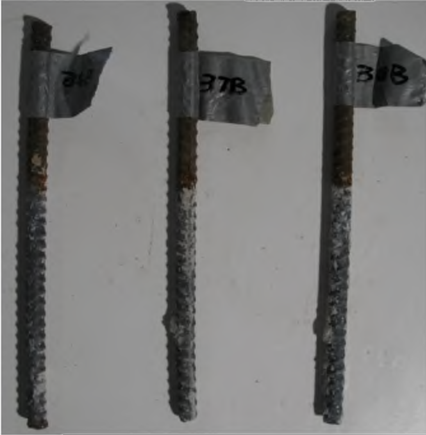
Figure 23 Black bars in ternary after impressed current test
