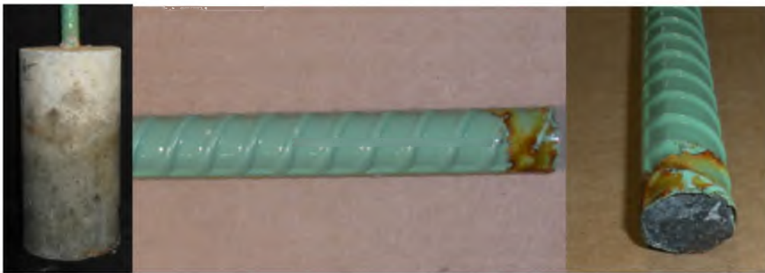
Figure 43 ECR (endcut) in OPC after impressed current test
