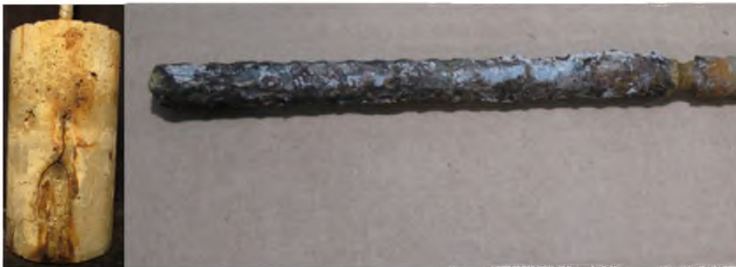
Figure 26 SSA in OPC after impressed current test
