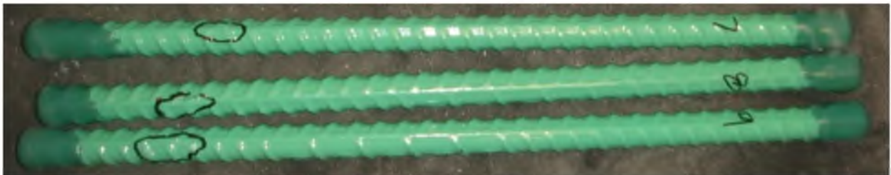
Figure 9 ECR bars with "mash" damage
