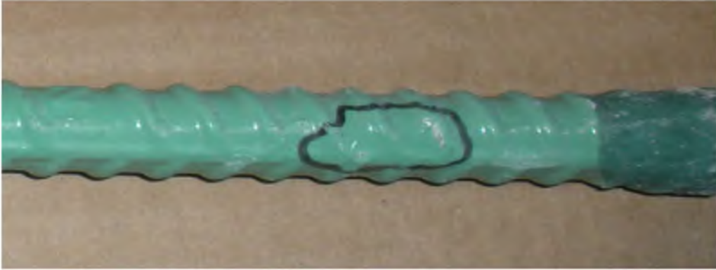
Figure 39 ECR (mashed) in OPC after impressed current test
