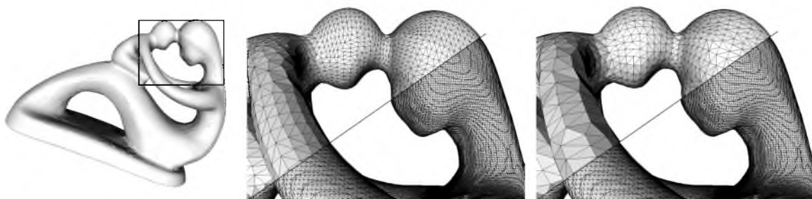
Fig. 7.11. Fertility model, 240K vertices, uniformly decimated to 16K vertices, 8K vertices. Our Fiedler approach is shown in the top-half image.
