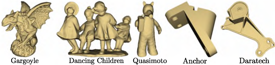
Fig. 3.3. Complex shapes created via our Polygonal MPU scheme. In our experiments, these shapes are utilized by performing synthetic range scanning under a wide variety of typical use-case scan parameters. This class of shapes contains many interesting characteristics for scanning, such as multiple scales of detail, nontrivial topology, and sharp features.
