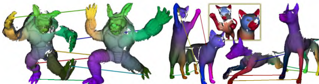
Fig. 6.10. Correspondence results across several different animal categories. In the inset, we depict the differences in the signature m_t(\mathbf{x}, \mathbf{x}) , color-mapped across the two shapes. Note the signature’s insensitivity to the lack of data.
