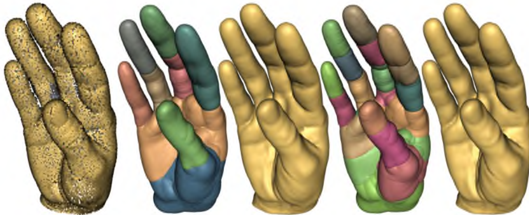
Fig. 5.15. From the point cloud on the left, we show segmentations of different cluster sizes, and the reconstructions. Note the insensitivity to the number of clusters.
