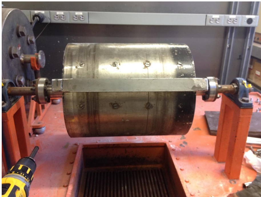
Figure 3.4. Counterweight to neutralize variation in center of gravity due to presence of steel handles.
