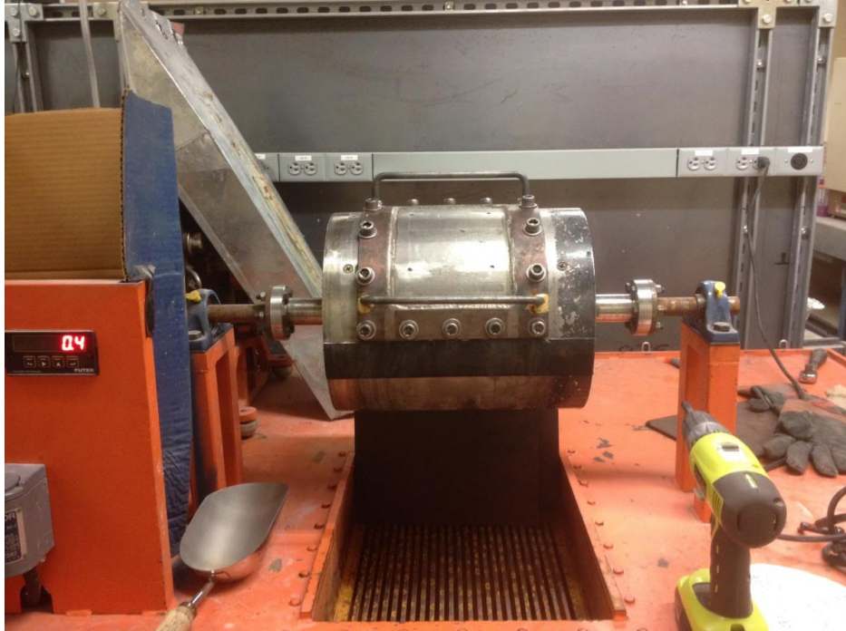
Figure 3.5. Illustration of torque meter coupled to the mill shaft.
