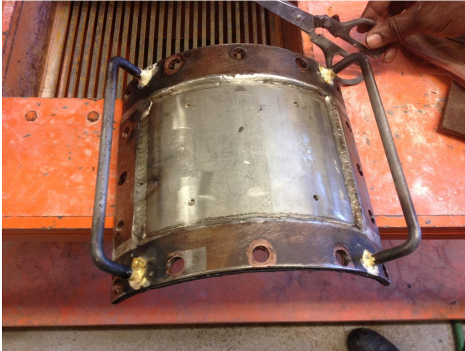
Figure 3.3. Mill shell replaceable cover plate with stainless steel handles.
