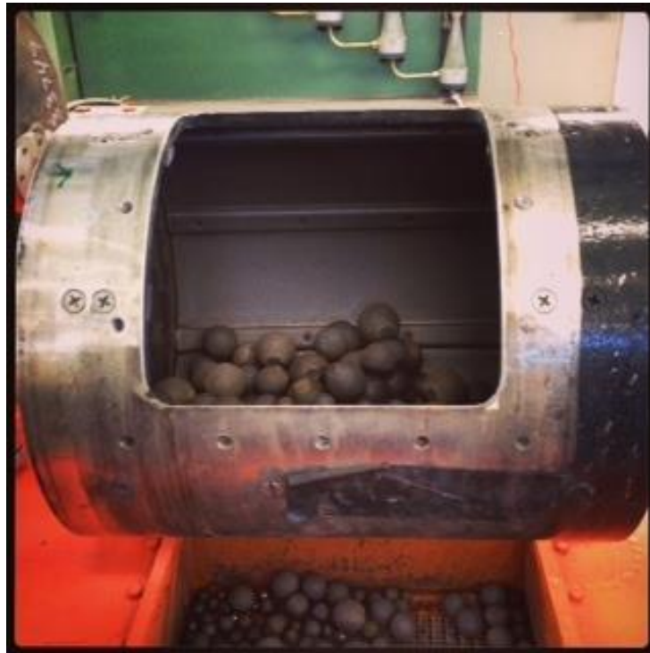
Figure 3.1. Partially loaded 10-inch batch grinding mill depicting square lifters configuration.
