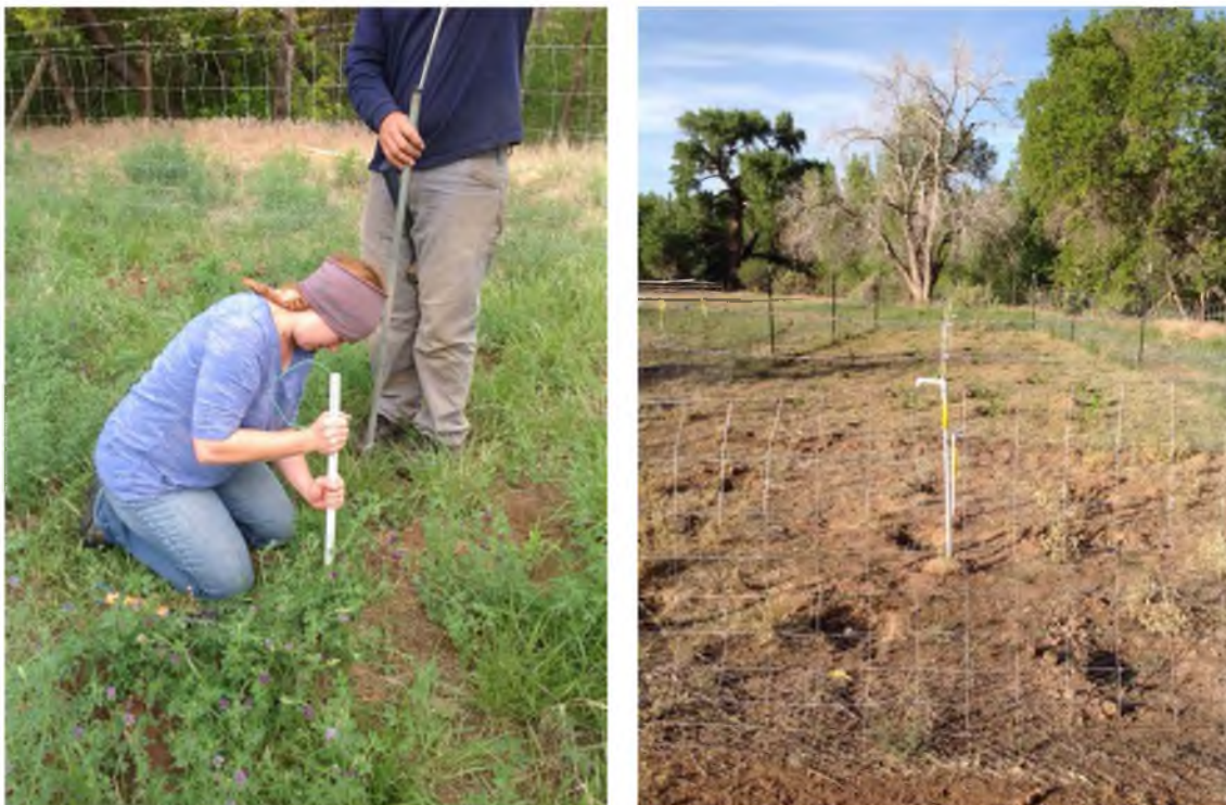
Figure 2-3. Photographs showing the placement of the soil sensors in the experimental plots (left) and an overview of the experimental plots taken facing south, showing sensors aligned down the center (right).
