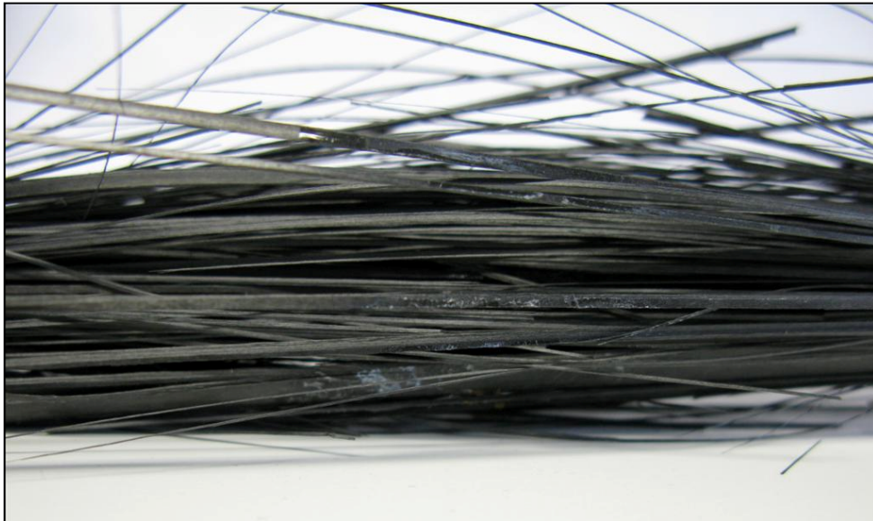
Fig. 3.12 – Failed CFRP rod from generation III anchor
