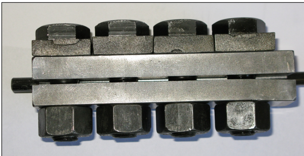
Fig. 3.14 – Clamped generation IV anchor showing increased width of outer slot from left to right
