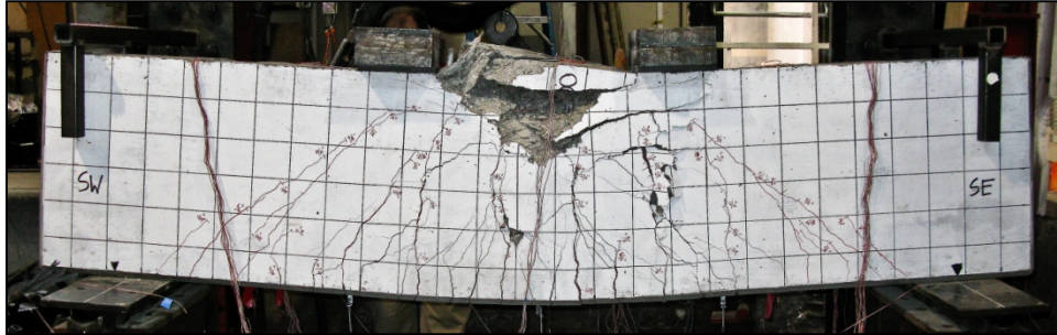
Fig. 4.9 – Failed specimen RST8 (repaired)
