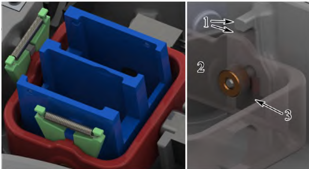
Figure 3.7: Close up views of spring return mechanism and tactile switch under gimbal. (1) Extrusions that the spring return arms align (2) Gimbal ring (3) Tactile switch
