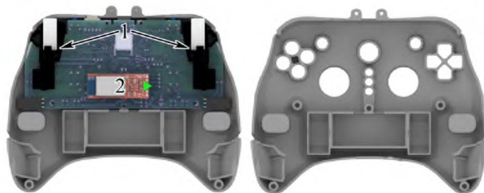
Figure 3.11: Back view of back-tactor controller with back shell removed. (1) Analog triggers (2) Optional Bluetooth module
