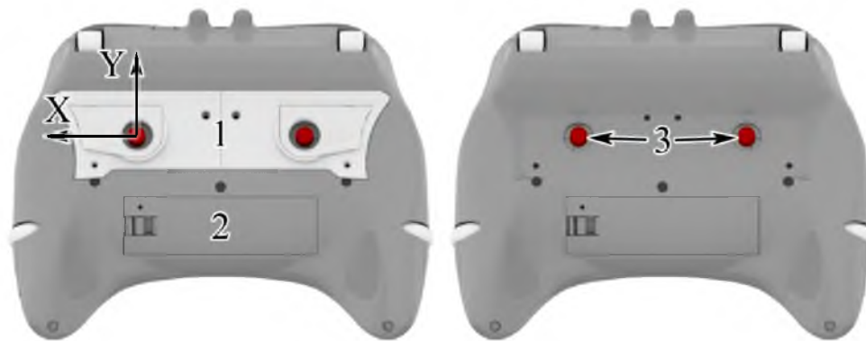
Figure 3.10: Back view of back-tactor controller with tactor axes labeled. (1) Removable finger restraints (2) Battery compartment cover (3) Tactors
