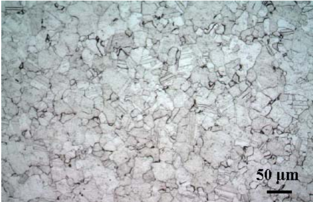
Figure 4.5 Optical micrograph of unseeded René 88DT grain structure. 200X
