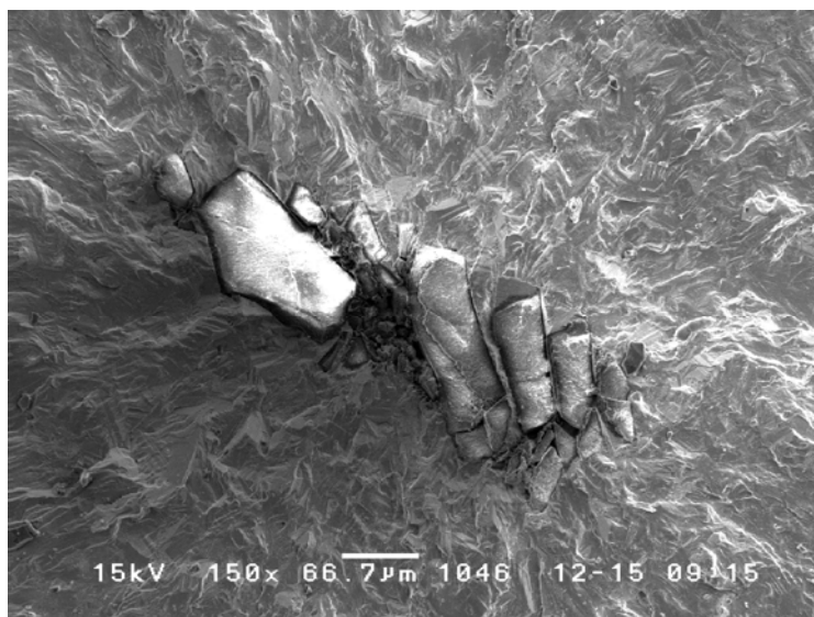
Figure D.18. Failure from internal-initiated seeded inclusion in specimen SD1-L18 tested at 640 MPa giving a life of 453361 cycles.
