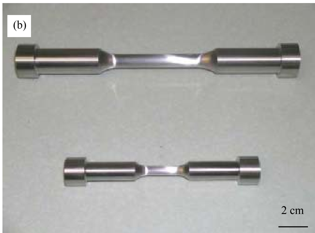
Figure 4.1 The button head specimen used in this study (a) Specimen geometry. All dimensions are in inches (b) Photograph showing a large and a small specimen
