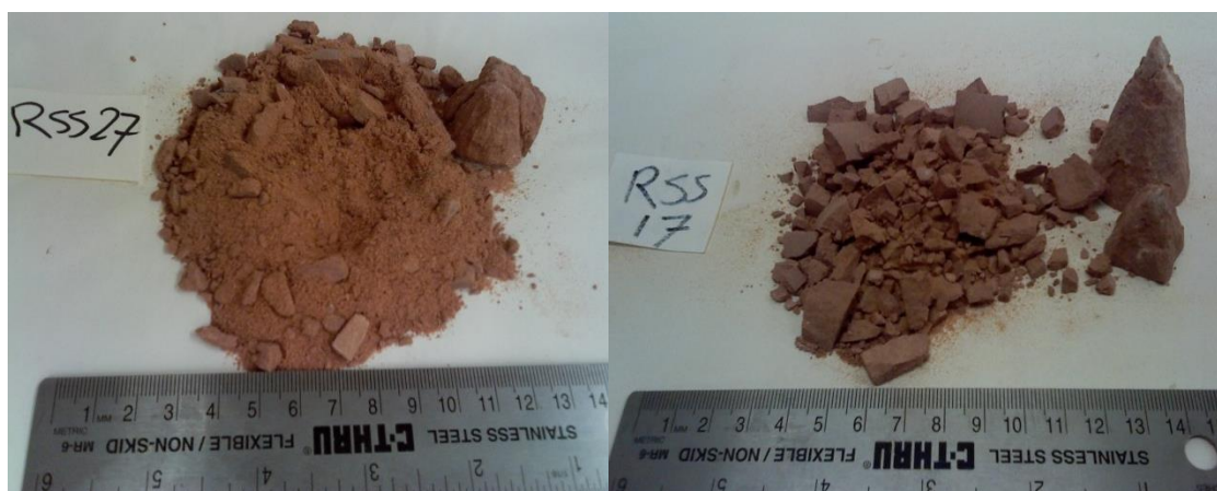
Figure 4.42 Fragment of samples of red sandstone (left: Saturated; right: Dry sample).
