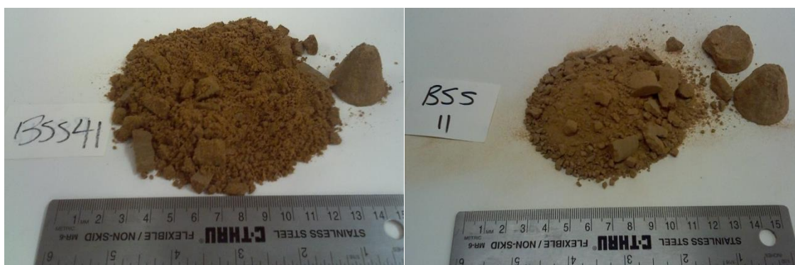
Figure 4.41 Fragment samples of buff sandstone (left: Saturate; right: Dry sample).
