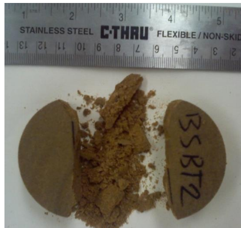
Figure 4.25 Buff sandstone disc after dynamic tension test by SHPB.
