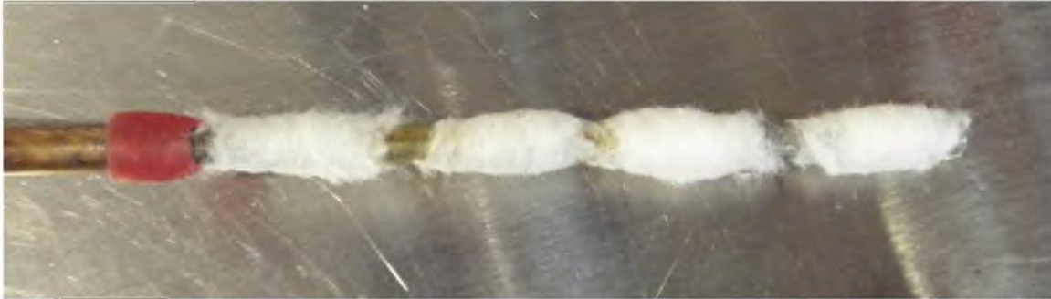
Figure 3.4: Thermal packers made from cotton, super glued to brass tubing with a silicon plug.
