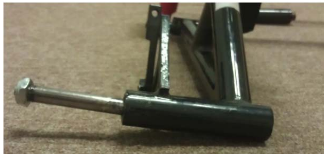
Figure 11: Bent Swing Arm of the Phoenix 1.5 (Densley, 2011)
