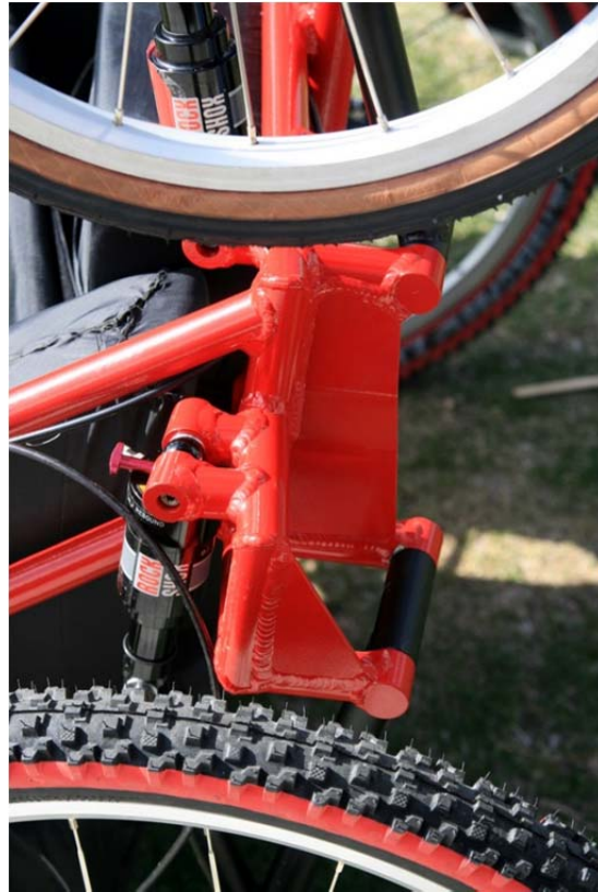
Figure 20: Shock Mounts and Gussets (Densley, 2011)
