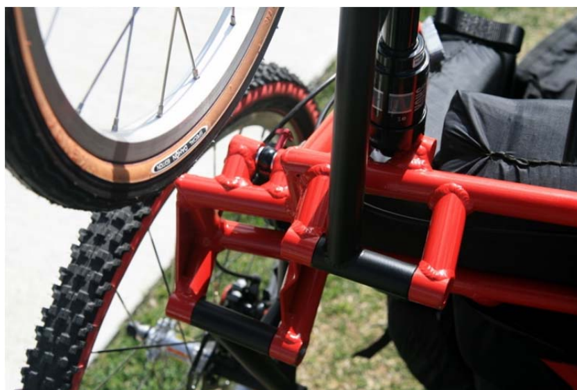
Figure 18: Swing Arm Attachment Location (Densley, 2011)
