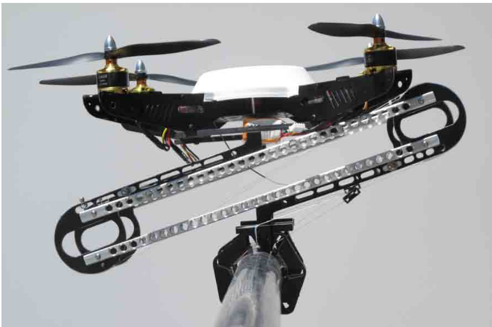
Figure 3.1. Quadrotor perching on a cylindrical railing. The landing gear is actuated by the weight of the quadrotor and creates a grip strong enough to withstand small-to-moderate environmental disturbances.
