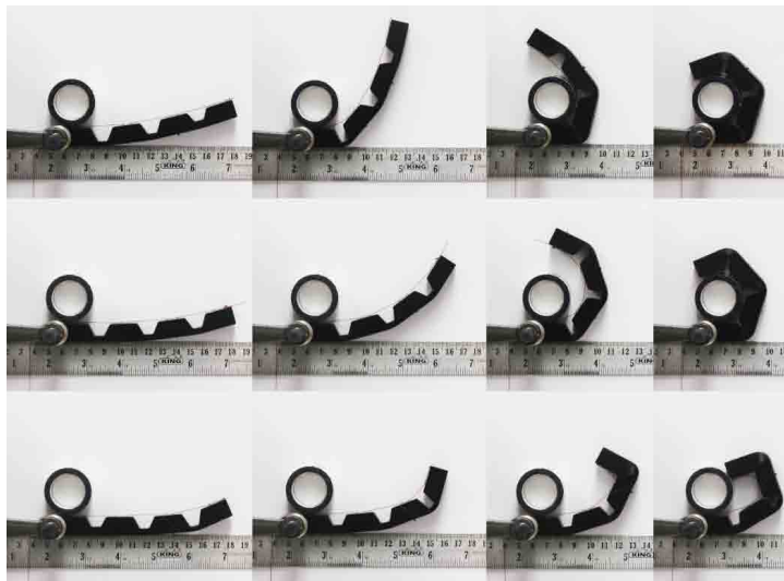
Figure 2.5. Depiction of how joint stiffness patterns affect form closure. (Top row): K_1 < K_2 < K_3 ; (Middle row): K_1 = K_2 = K_3 ; (Bottom Row): K_1 > K_2 > K_3 .
