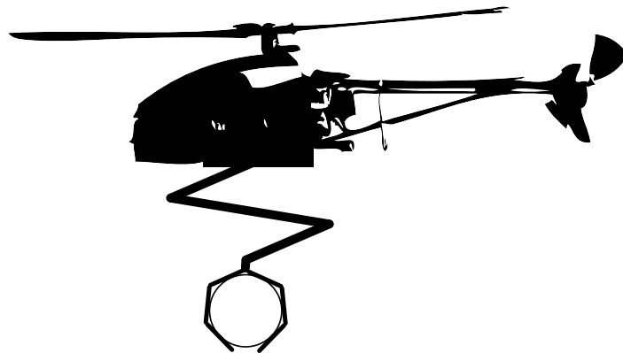
Figure 1.1. Conceptual drawing of perching mechanism. Through the use of clever mechanism design, a rotorcraft (e.g., helicopter) can passively perch on a curved surface, similar to a bird.
