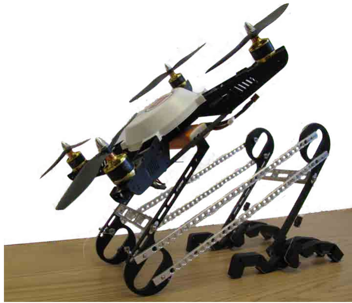
Figure 3.13. Landing on flat ground. The system reaches a stable position resting on the feet and knee joints.
