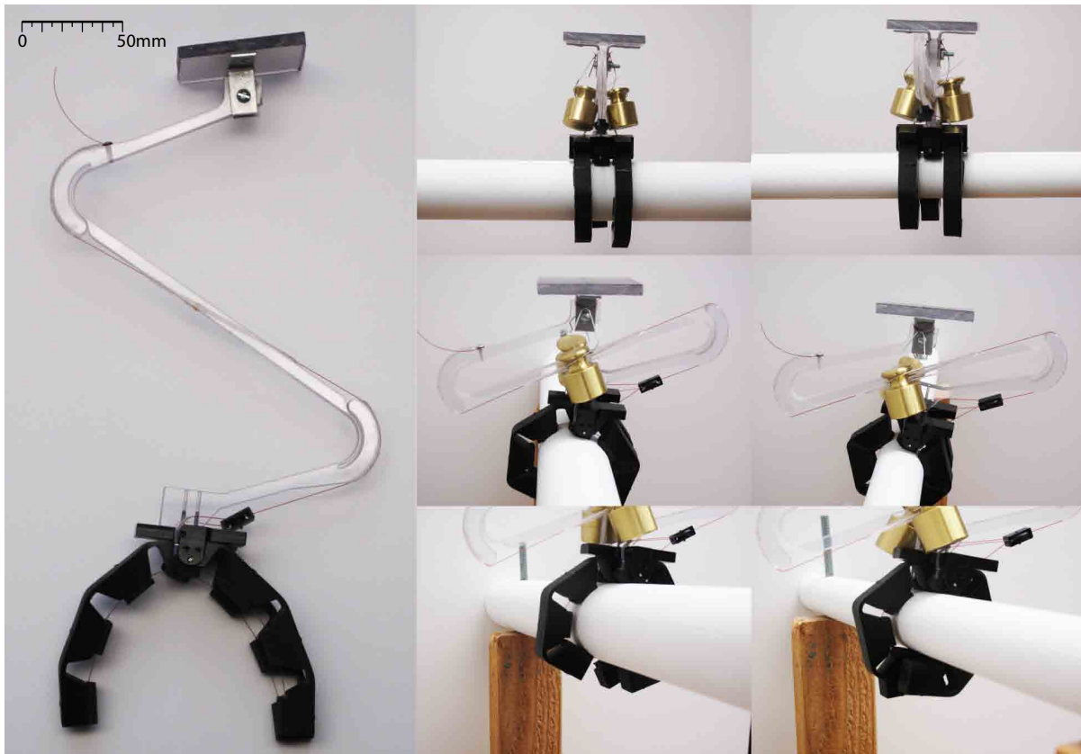
Figure 2.10. Demonstration of functional prototype. (Left column): Image of landing gear in its relaxed state. (Center column): Series of images showing a successful perch on a rod of diameter of 49 mm. (Right column): Series of images showing a successful perch on a rod of diameter of 33 mm.
