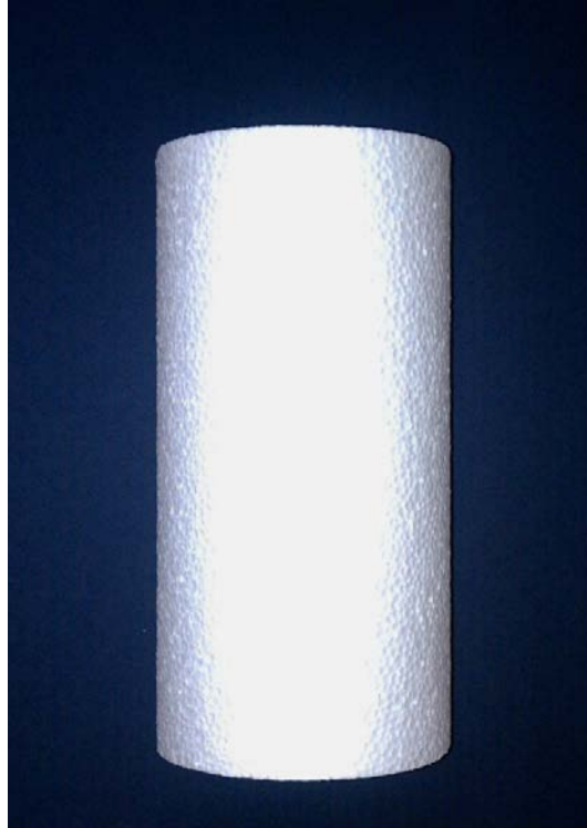
Figure 1: A 10 cm diameter 20 cm height (2:1 ratio) cylindrical sample of EPS geofoam.
