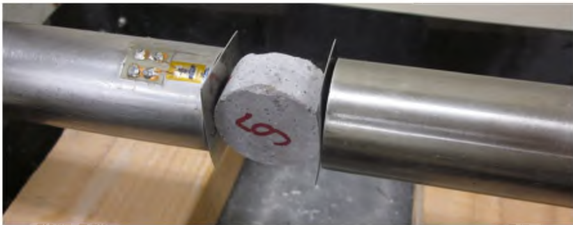
Figure E.13 Brazil test specimen in SHPB
