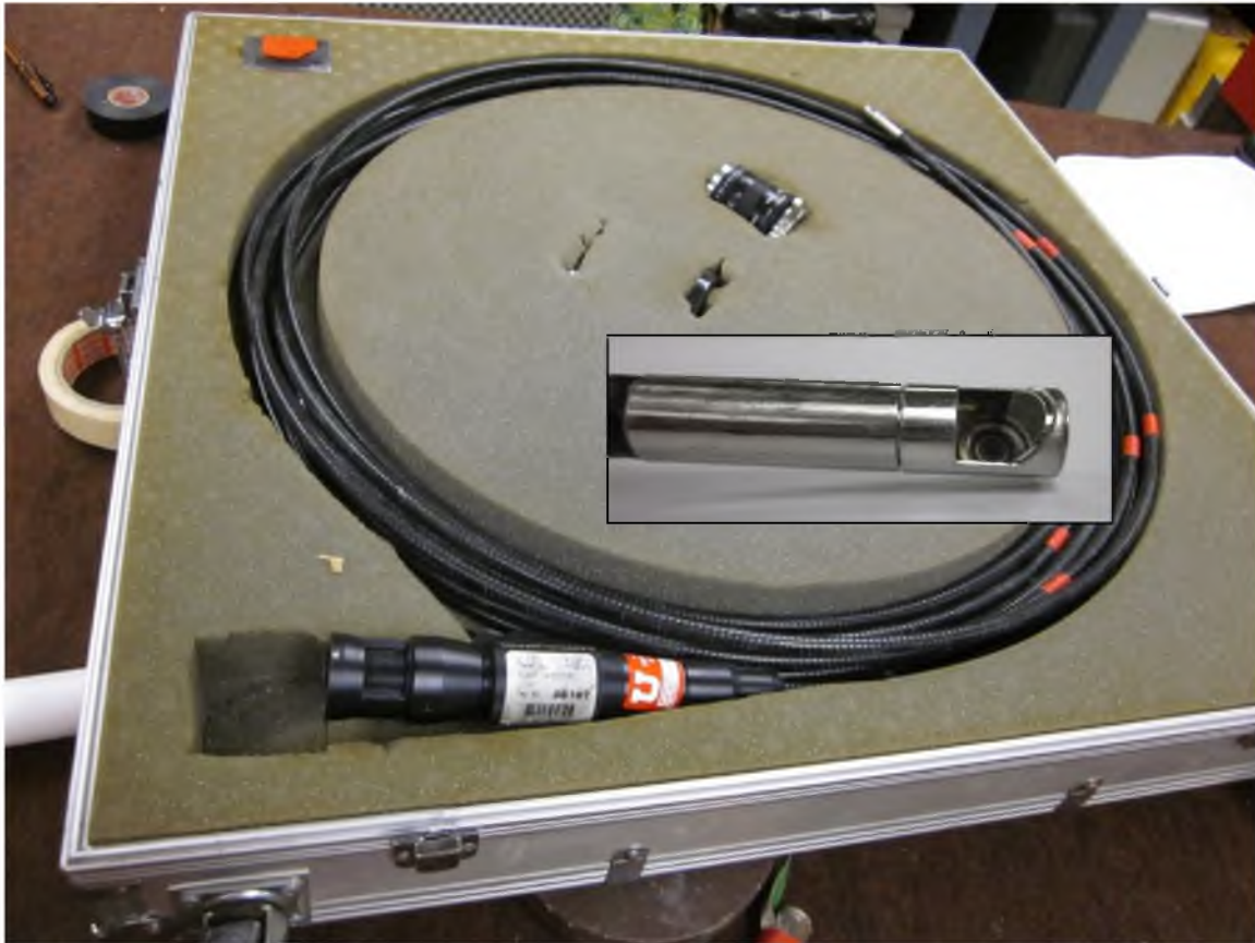
Figure 3.11 Borescope; viewing aperture inset
