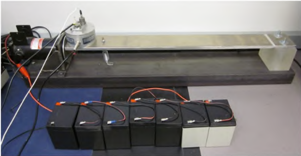
Figure 3.4 Apparatus for testing vibration transducers
