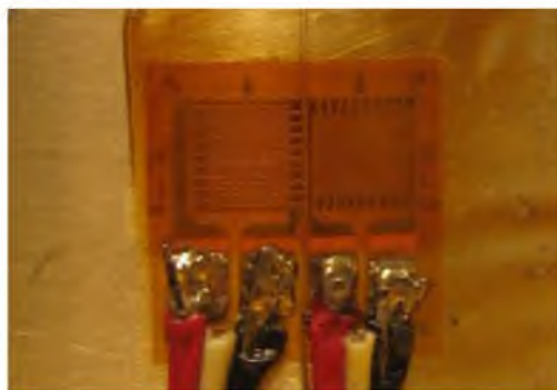
Figure C.1 Two strain gauges, here mounted in perpendicular orientations
