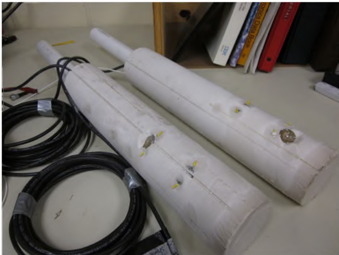
Figure 3.14 Vibration transducers precast in Hydro-Stone™
