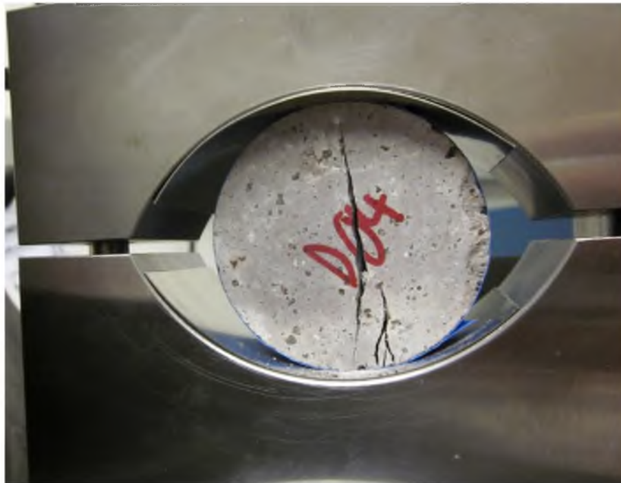
Figure E.2 Specimen after failure in Brazil test
