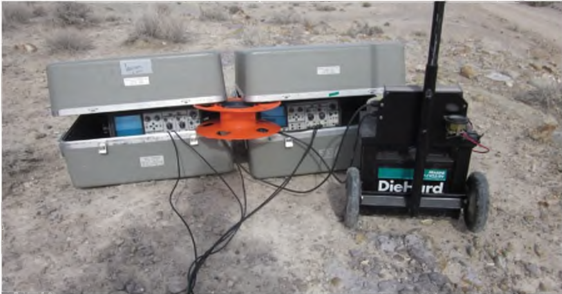
Figure 3.17 Oscilloscopes in their protective covers, powered by a deep-cycle battery hole collar and joined with another length of nonelectric initiation tube, which was connected to the external trigger for the oscilloscopes.
