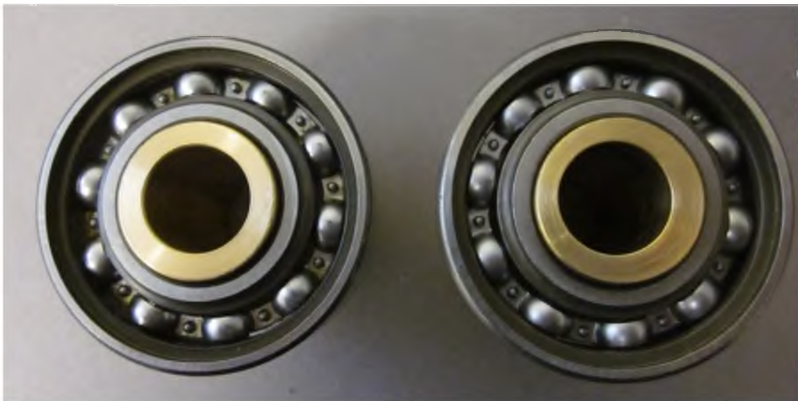
Figure 3.5 Offset cams 6.096 mm (0.024 in.) (left) and 12.70 mm (0.050 in.) (right)
