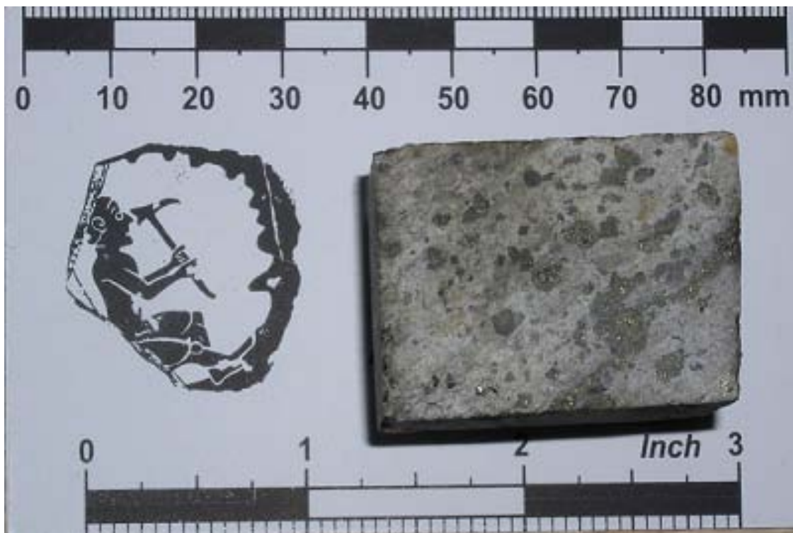
Figure 5.1. Sample K01 contains disseminated pyrite (size: about 2mm). Monzonite from the Kori Kollo mine, Bolivia.
