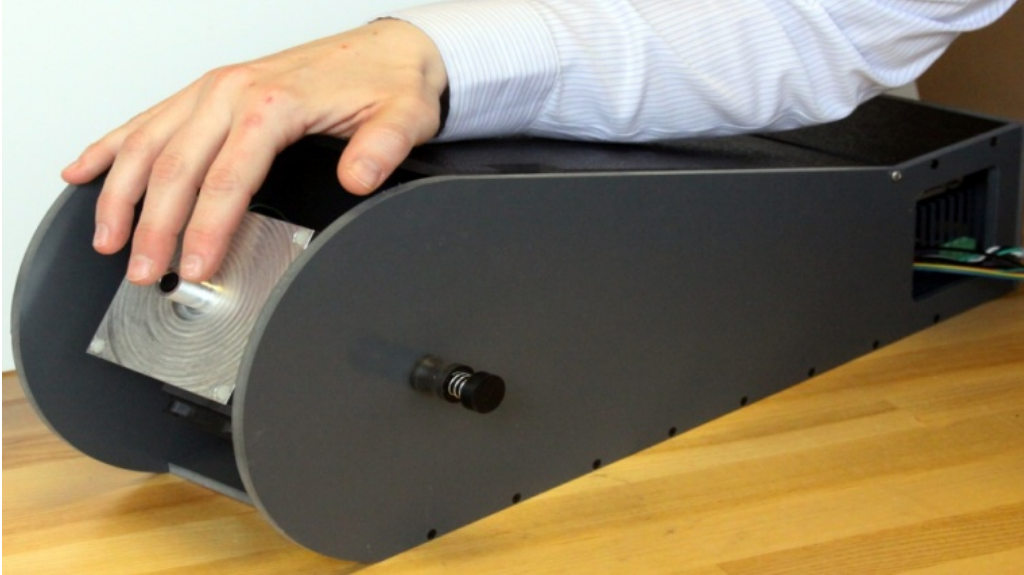
Figure 5.1: The Vibrotactile Threshold Evaluator for Workplace Screening (VTEW) device with a subject's arm (cover removed to show the surround and the probe).
